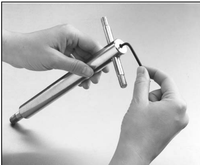
Figure 10. Tightening setscrew with hex key.
